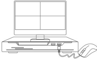
When connect the camera system without Internet, you can preview, playback or change settings on monitor by using the mouse.
