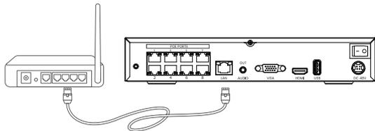
1b. If you want to operate the security camera system in a closed environment, do not connect the LAN port to your router.
