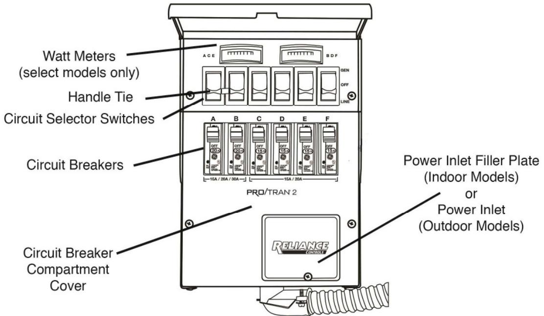
**Circuit breakers.** Each transfer switch circuit has a 1-in interchangeable circuit breaker that protects the branch circuit when the circuit selector switch is in the GEN position. In the LINE position, each branch circuit is protected by the breaker in the load center.
