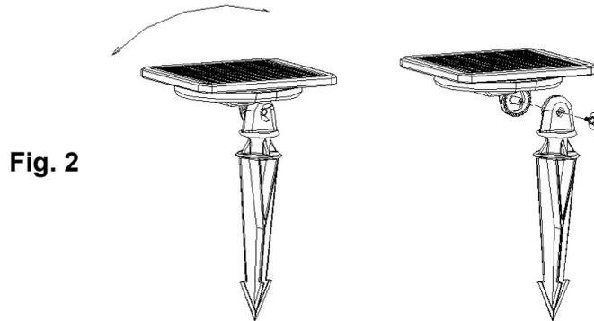
1. To install the solar panel in a remote location, unwind the extension wire under the solar panel to the desired length.
