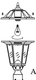
1. Attach Part (A) to the bottom of the fixture by twisting clockwise.
