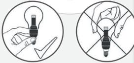
**Note:** Make sure the lens is fastened securely.
