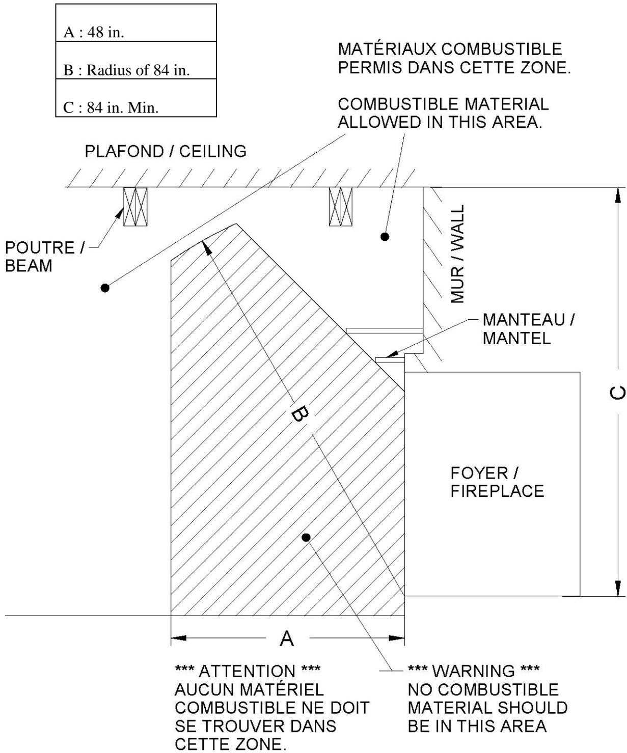
Figure #17: Installation of Fireplace Facing
