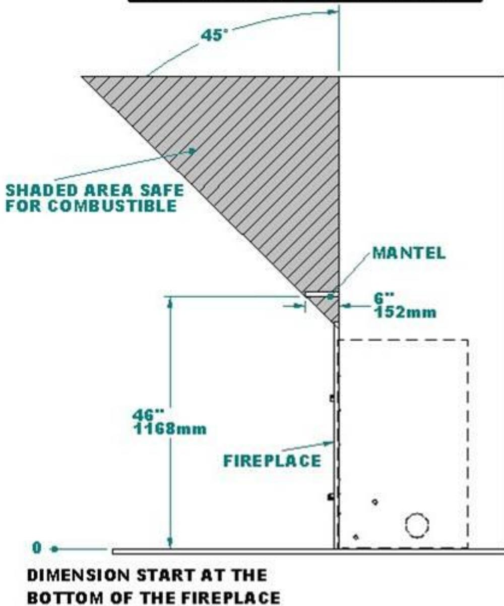
Figure 16b : Combustible material positioning
