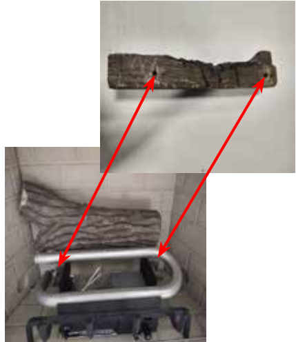
Figure C - Middle Log Placement
