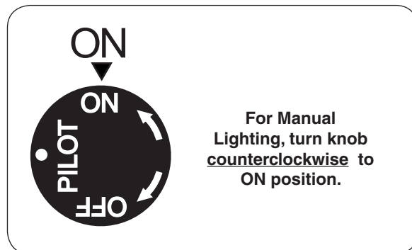
Fig. 13-1 Control knob detail (ON) - pan models
