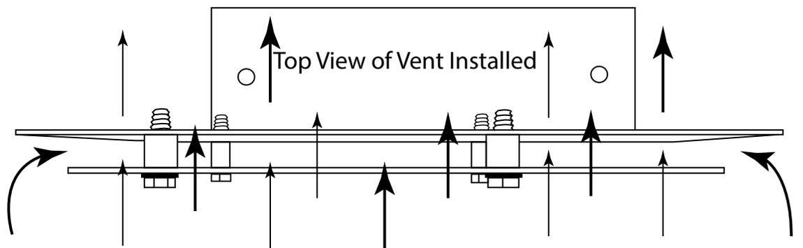
Air flows through and around the vent with the spacers installed to provide 18 square inches of cross ventilation for one side of the enclosure.
