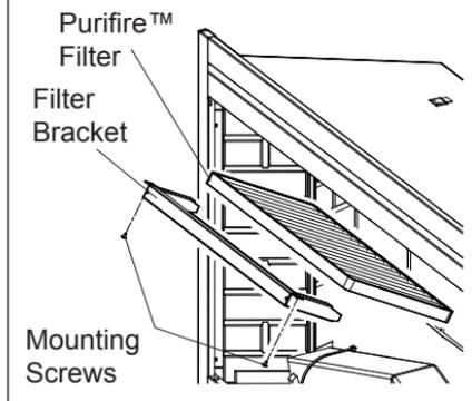
1. Remove the 2 mounting screws from the air filter bracket.
