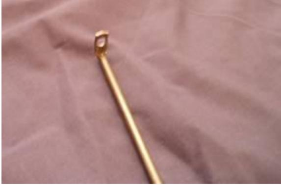
Both rods have a flat end; using a pair of vise grip pliers, very gently bend each flat end at a ninety degree angle. This will enable you to attach the rods directly to the side of your fireplace opening. *If you are installing the rod kit using the secondary bracket for arched fireplaces, leave these ends flat.*
