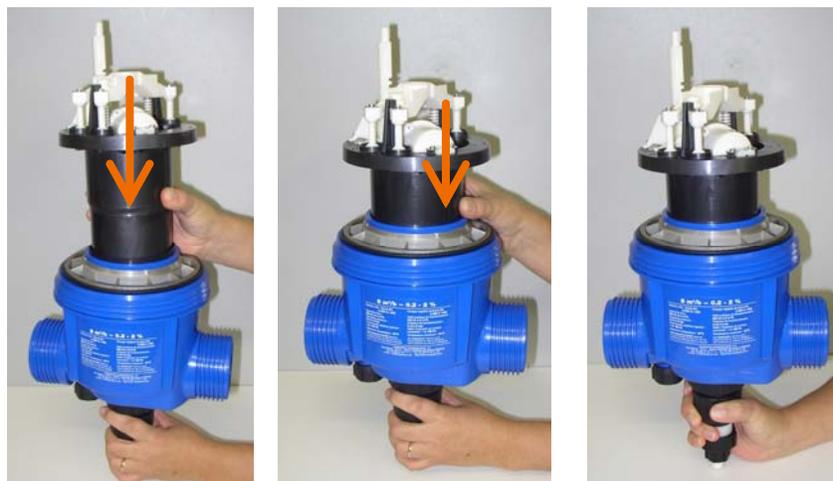
Insert the lower part of the piston half way down the body. Then let go of the piston. The piston should be snug in the body and the piston should not fall in, if it does, the piston shell needs to be replaced. Also inspect the inside of the body and look for deep vertical scratches, if this is the case, the body needs to be replaced.
