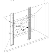
Step 3B: Attaching the mounting brackets to the monitor (spacers used due to recessed hole patterns)
