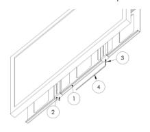
Step 4: Securing the mounting brackets to the wall plate
