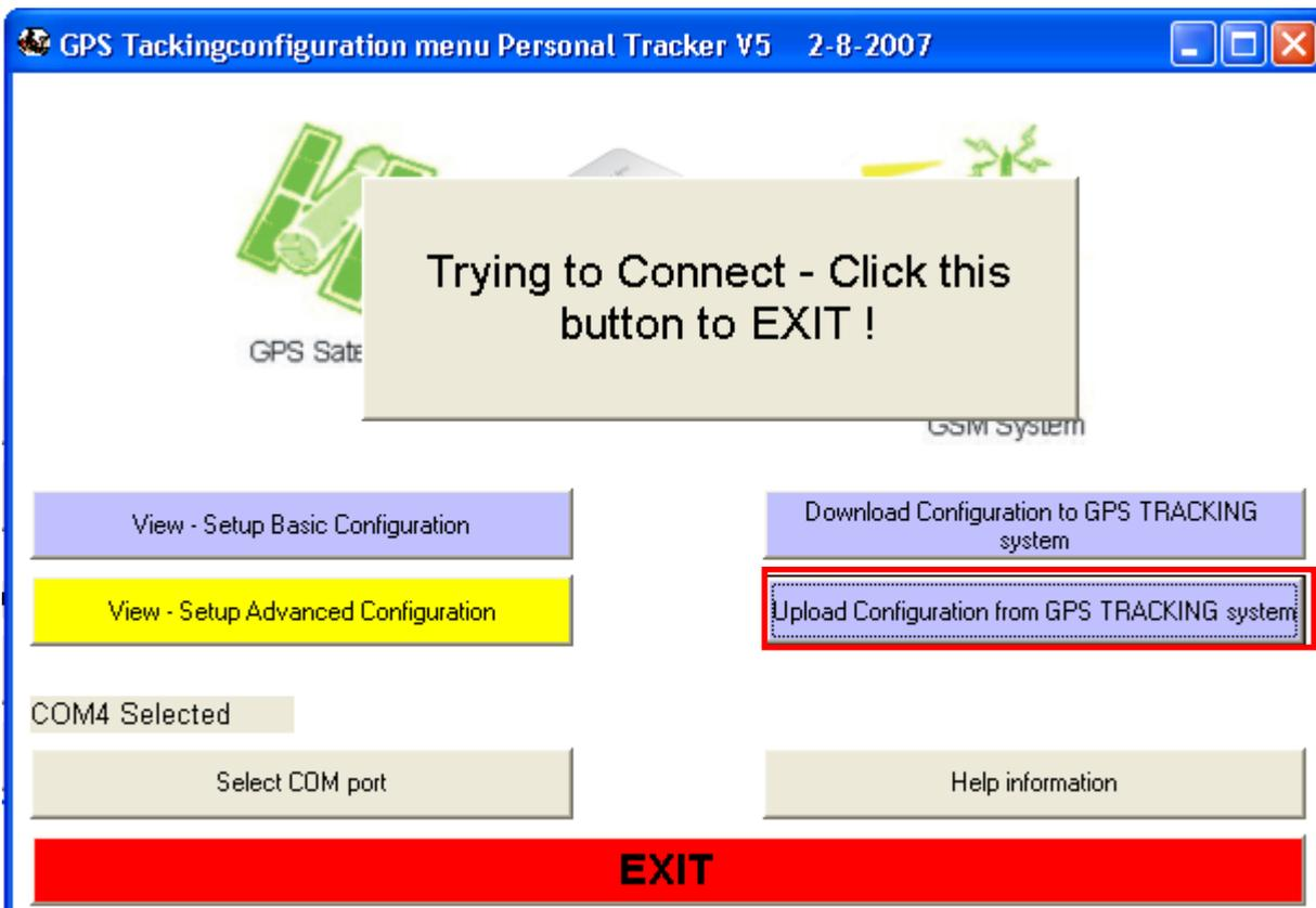
Always upload the current configuration from the WGAT first. This way it is easy to configure and the setup the unit. You must use the correct WGAT firmware version. The configuration file cannot be uploaded if the version is incorrect.
