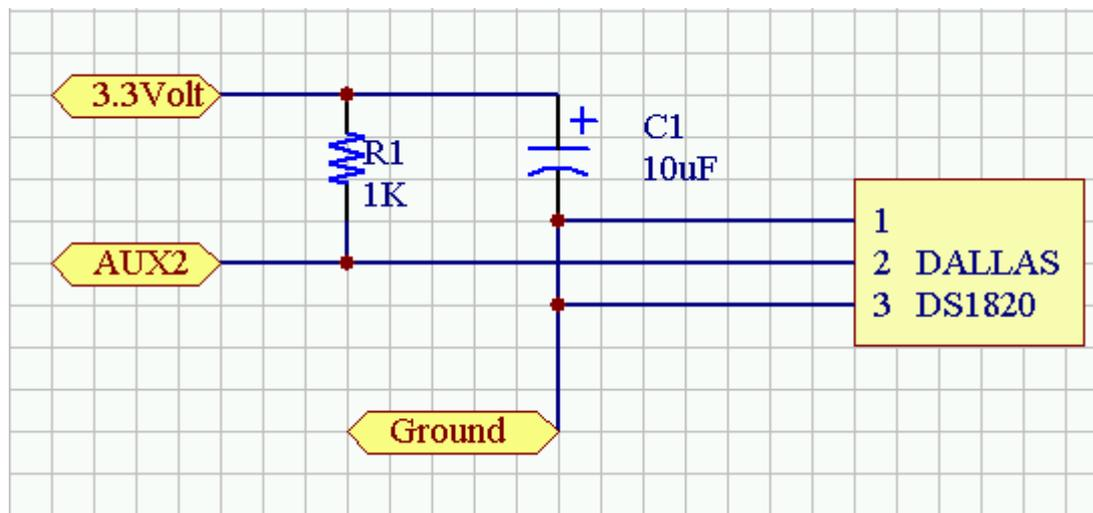
When the DS18S20 is connected as shown above and enabled in the configuration menu program the temperature measured is automatic included in every location message.
