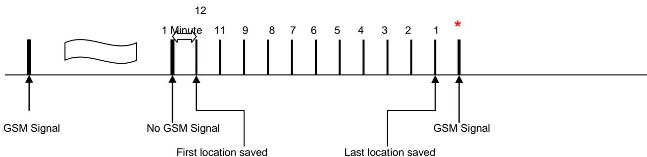
When the next real time tracking location (\*) needs to be sent back and the transmission is successful the WGAT will try to send back the missed locations. Missed locations are sent back starting from the last saved location (1). One message (SMS or GPRS) will contain 4 locations.
