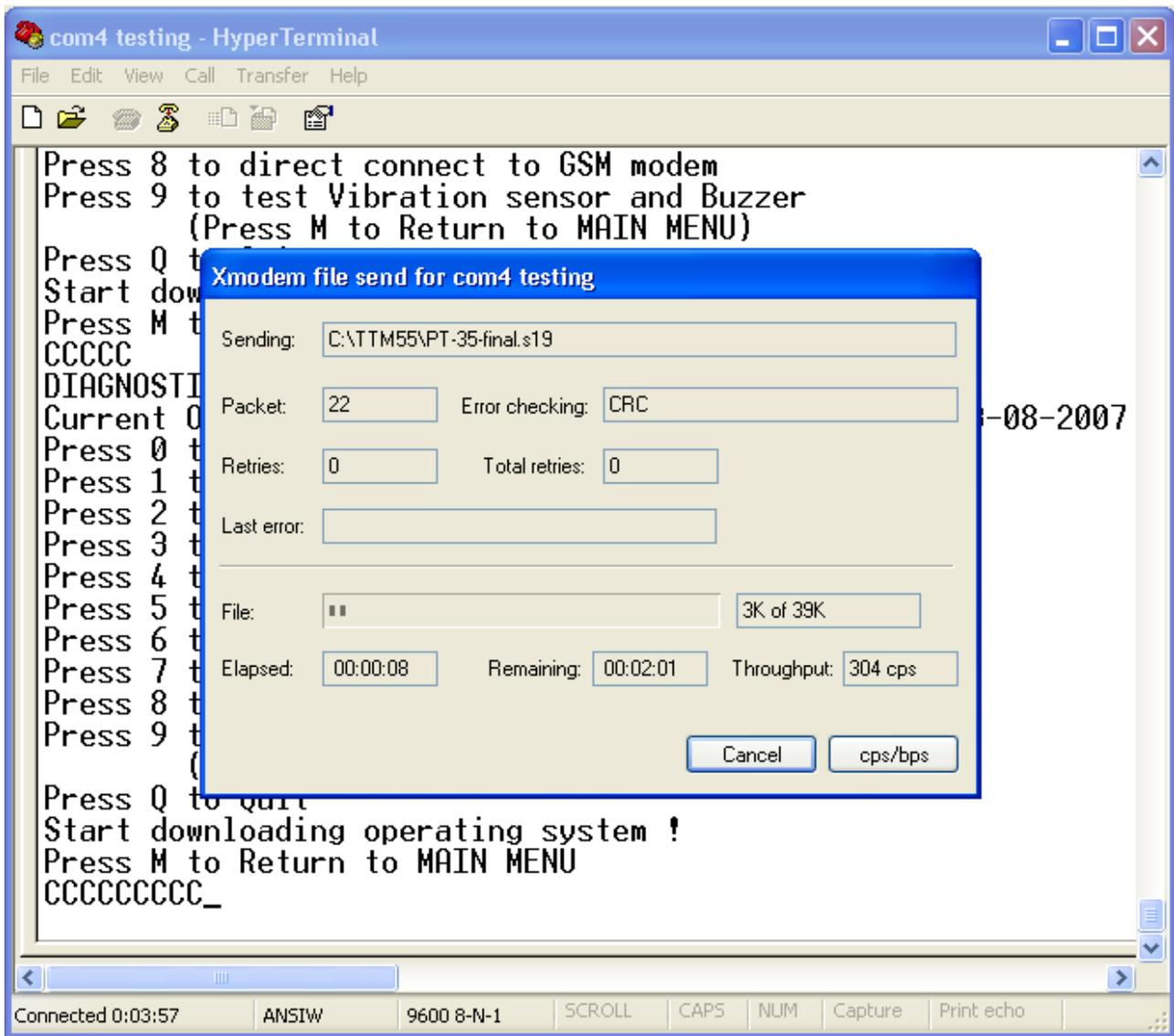
After upload the WGAT unit will restart into the **Diagnostic Main Menu**. The Version and Date details of the new Operating System will be displayed.
