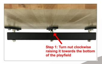
d. Next, begin to tighten the nut located just below the metal bar on the center. Make a few more turns. Now check the straight edge for improvement. If more adjustment is needed, continue tightening the bottom nut. Once you have reached the desired adjustment, tighten the nut against the top of the metal bar as described in step 4. Continue to the next climatic adjuster and repeat the above steps.
