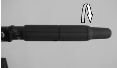
2. Move the Forward-Reverse switch to the desired direction position.
