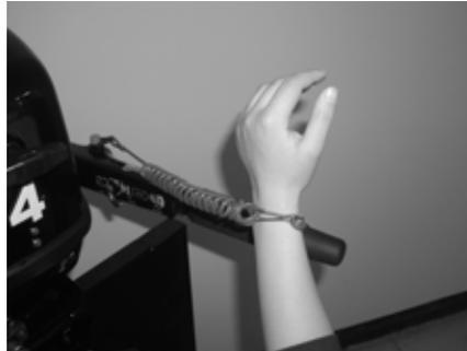
Always attach lanyard to clothing or wrist when operating the outboard.
