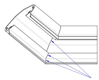
Weld underside of seams only
