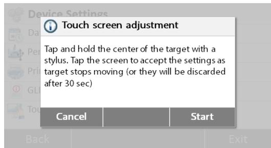
Press the **Start** button to start the adjustment.
