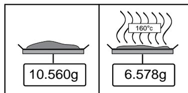
The Ohaus Moisture Analyzer comprises two instruments: a precision balance and a dryer unit. In contrast to other thermogravimetric methods (drying oven, infrared, microwave), the Halogen Moisture Analyzer operates with a halogen dryer unit. This ensures fast heating of the sample and thus guarantees rapid availability of the measurement results.
