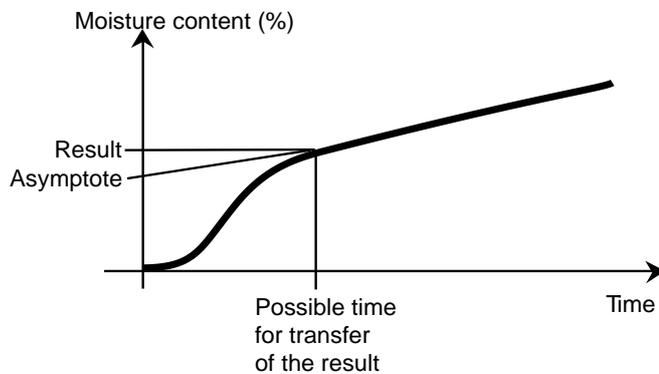
Measurement results of such a drying profile can be optimized:
