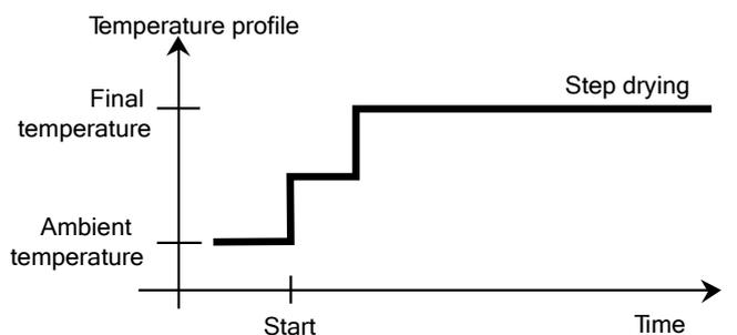
An alternate application possibility lies in the selective determination of the moisture at different temperatures. Gypsum, for example, releases only its surface water at 50°C,
