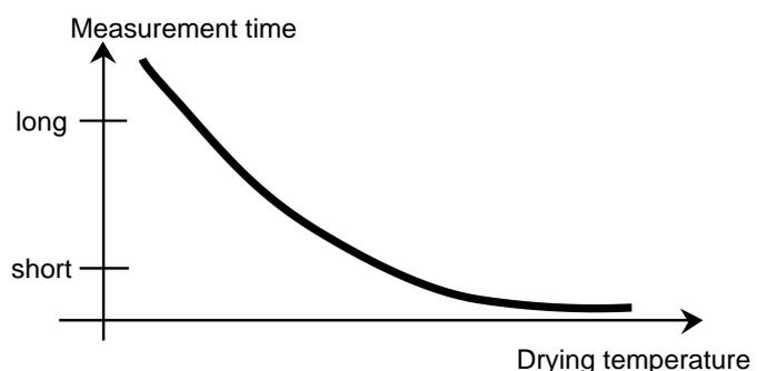
For MB120, OHAUS provides a temperature guide to estimate the proper temperature for reference. Please see section 9.2 for details.
