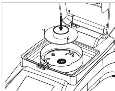
Press the **Start** to initiate the temperature calibration process. Follow the screen prompts throughout the process.
