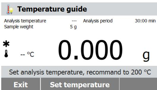
Press the **Set Temperature** button to enter the temperature setting.
