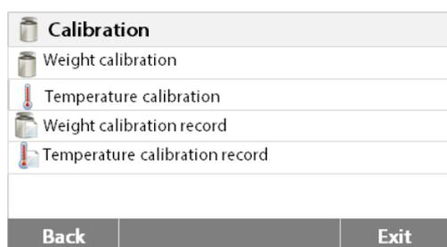
Press the Weight and temperature calibration button to access the calibration screen.
