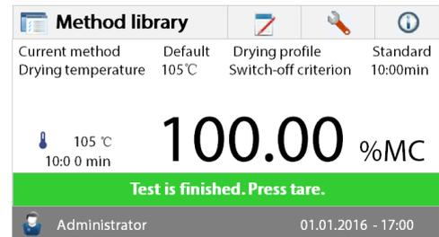
The display indicates the Method Name, Temperature/Time, actual temperature, elapsed time duration of the test, moisture and curve. The test automatically stops at the end of the measurement. If you want to end the test sooner, press the
