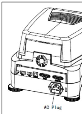
Connect the power cord to the power supply socket located at the rear of the Moisture Analyzer and to the power supply outlet. The Moisture Analyzer becomes operational as soon as power is applied. The display will remain off until the **On/Off** button is pressed.
