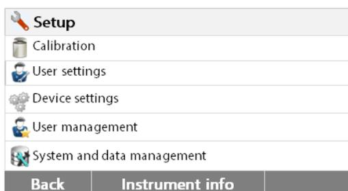
Press the Setup button to access the Setup screen.
