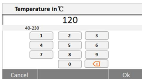
Enter the desired drying temperature and press the **OK** button.
