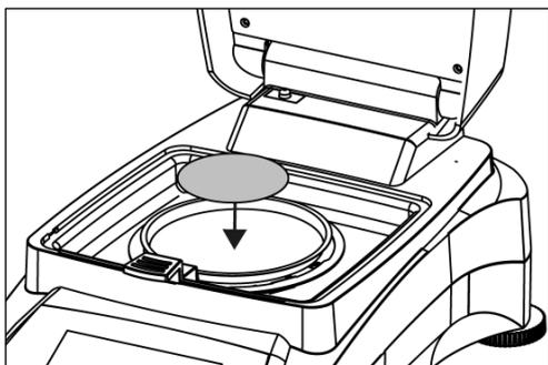
Place the empty sample pan and glass fiber pan in the pan handler. The sample pan must lie flat in the pan handler.
