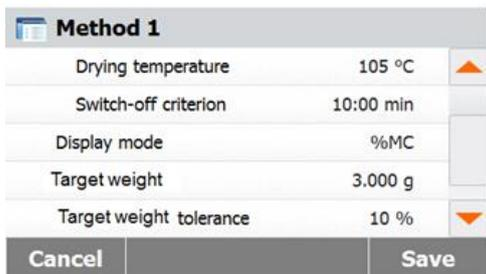
Press **Target weight tolerance** to set the tolerance of the Target weight.
