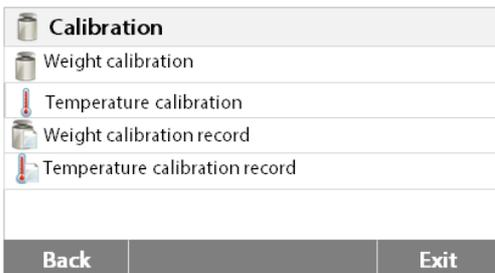
Press **Weight calibration record** to list the weight calibration record data.
