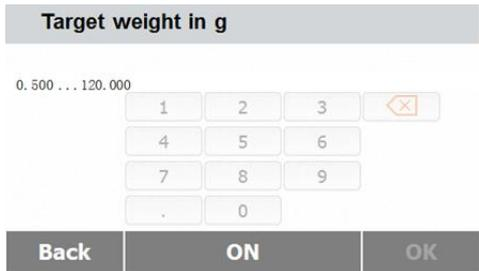
Enable the Target weight and press the **ON** button.
