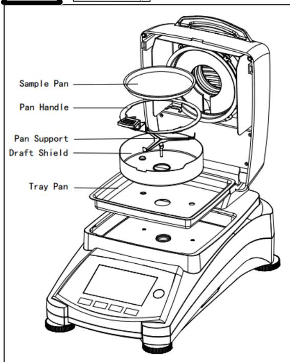
Open the cover and remove the pan handler, sample pan, draft shield, and heat shield from the instrument before cleaning.
