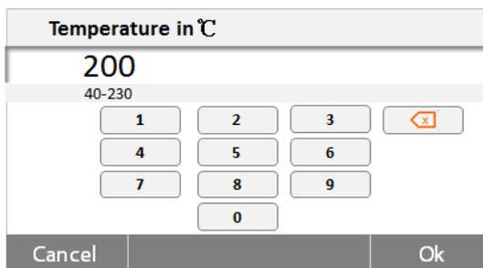
Set the temperature. We recommend to not set it above 200°C. Press the **Ok** button to save the temperature and access to next step.
