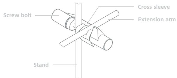
Check that the stirrer is held in position firmly prior to each use and also at regular intervals. The position of the stirrer must only be adjusted when the equipment is stationary and the power supply is disconnected.
