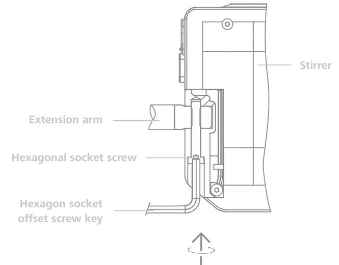
Ensure that the extension arm is fitted securely. Vibration may cause the screw to become loose. It is therefore necessary for safe use to regularly check that the extension arm is attached securely. Tighten the hexagonal bolt as required.
