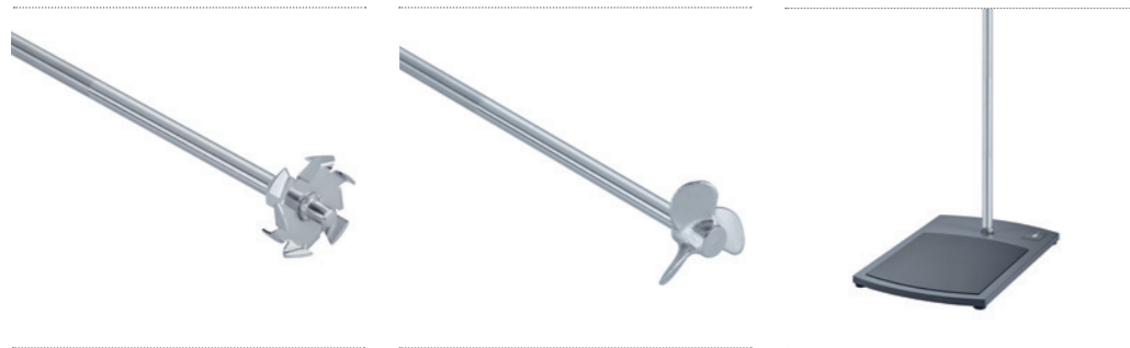
R 1303 Dissolver stirrer Radial flow, for drawing the material to be mixed from the top and bottom. High turbulence, high shearing forces. Particle reduction. Used at medium to high speeds. Ident. No. 0002746700
