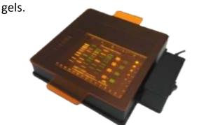
Orange filter cover placed for gel viewing
