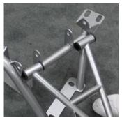
\*Now you can slowly rotate the other end of the A- arm towards the back slot of the K-member. Stay well below the mounting bolt holes.
