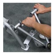
Now you can pull rear side of the A-Arm in place to align with mounting bolt holes.
