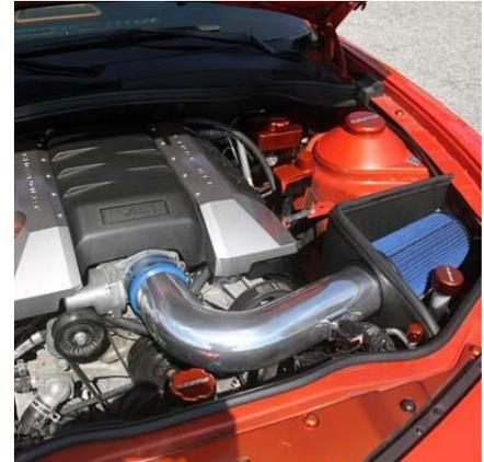
Install the weather stripping along the stop of the air shield, plug in the mass air sensor. Go back and tighten the clamps on the throttle body to intake tube. Check all connections and re-install the engine cover.
