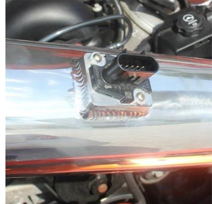
Remove the factory Mass Air Sensor from your stock air intake and install into the new air intake tube making sure the arrow is pointing towards the throttle body. This is a directional sensor.
