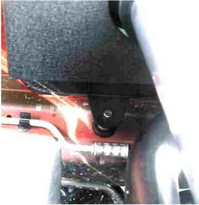
Installing the shield make sure the stand off goes into the factory rubber grommet first then line up the second tab with the stud on the other side.
