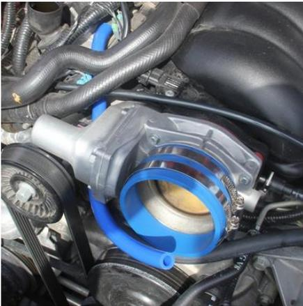
Route the provided vent hose to the vent tube on the valve cover and shown. Use the provided clamp on the vent tube to hold it in place.
