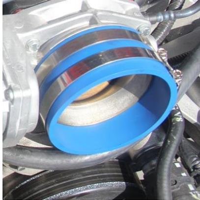
Slide the silicone coupler over the throttle body with the 2 4" hose clamps, tighten the back one onto the throttle body and leave the other loose for now.
