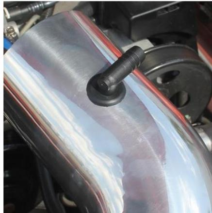
Insert the rubber grommet into the air intake tube followed by the plastic elbow. This is the connection for the vent hose. Slide the air intake tube onto the coupler for the throttle body and push the vent hose onto the fitting.
