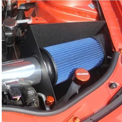
Install the nut over the stud on the back side of the air shield then slide the other 4" clamp over the filter and push the filter onto the intake tube. The rubber neck of the filter should go through opening in the air shield, then tighten down the filter clamp.
