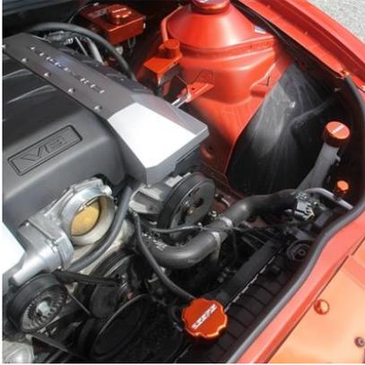
Start by removing the factory intake tube, vent tube and air filter assembly.
