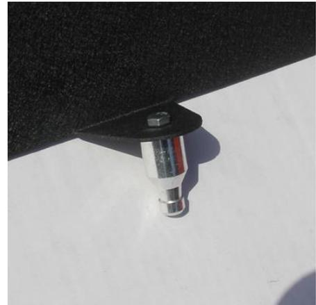
Install the stand off onto the air shield as shown with the provided bolt.
