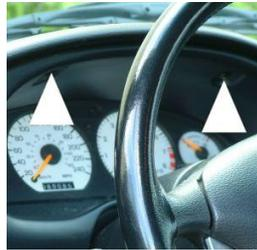
Using a torx screwdriver, remove the two bezel retaining screws from the top of the dash bezel. Once removed, gently pull on the bezel which will pop away from the dash. When the bezel has been removed, remove the four speedo cluster retaining screws. Tilt the cluster outward and detach the two Electrical plugs by depressing the tabs on the top. The speedo cluster should now be able to be removed entirely from the dash.
