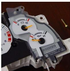
Carefully slide each piece of the Gauge set over top of the factory needles. **DO NOT REMOVE THE NEEDLES!** Repeat the same procedure for each piece. For 1999+ Mustangs the gauge set is one piece, but the same procedure applies.
