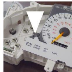
On 1994-1998 Mustangs the left gauge assembly must be removed to install the center overlay. Use a flat screwdriver to pry the gauge assembly out of its sockets. It will simply pop out. Route the overlay electrical wire between the gauge assemblies as pictured, and reinstall the assembly.
