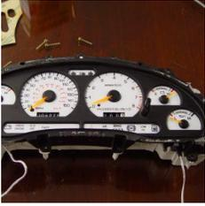
Re-install the black / clear bezel and the gold retaining screws.
