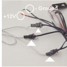
Plug each wire connector to the supplied transformer. There is no specific connector required, and there will be transformer plug left over for a future product.
