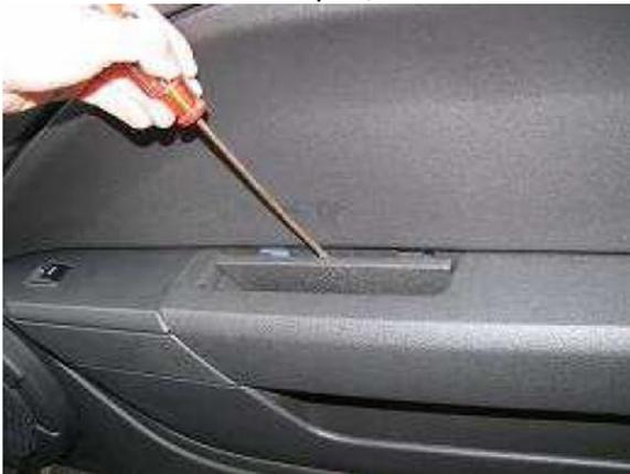
5. Remove the window switch plate assembly by prying up the top cover and gently pulling out the entire switch assembly almost horizontally. Remove the plugs from the switches and remove the assembly.
