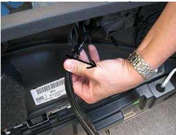
11. Remove the cable and the spring inside the stock handle. Remember the orientation of the spring, which will be re-used with the new handle.
