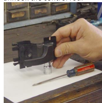
Turn the handle clockwise to unhook the control rod.
