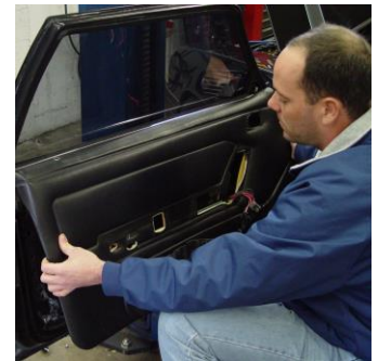
Carefully lift the inner door panel off of the door.
