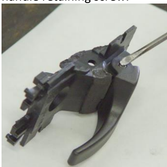
Remove the Phillips door handle retaining screw.
