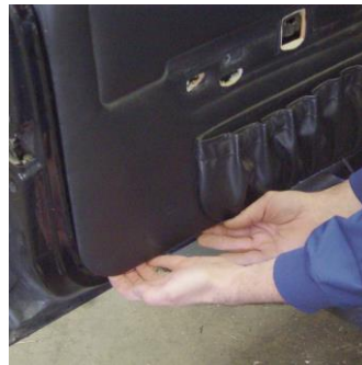
Remove the retaining clips on the lower part of the inner door panel.
