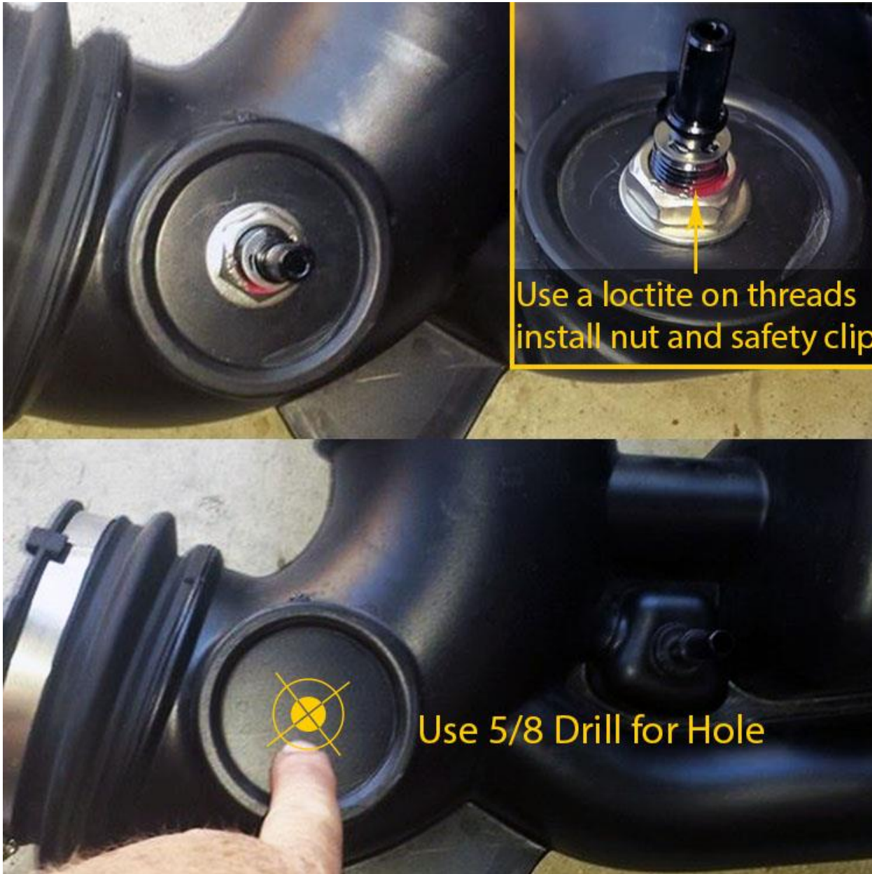
UPR Plug n Play WOT Fitting Installation
