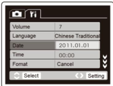
2. Under recording or photo mode, press "MENU" to enter the setting mode. Press "up"
