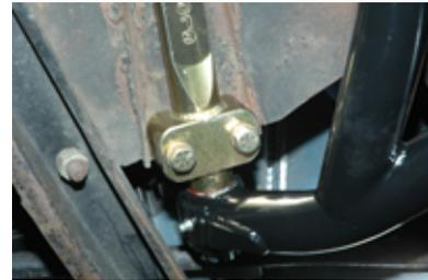
9. Install the 7/16 bolts towards the front of the shaft using new bolts and washers. Reuse the factory-threaded block.
