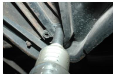
7. Remove the lower control arm from the frame.
