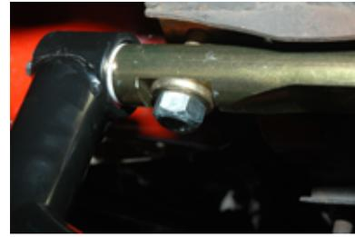
8. Install the new lower control arm with new hardware supplied in your kit. The 9/16 bolt supplied in the kit requires using two thick washers, one on the top of the frame and one next to the shaft. Place one thick washer on a 9/16 bolt, install from the top down through the frame.
