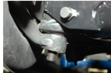
12. Slowly raise the arm to fit the ball joint into the spindle. Install the castle nut on the ball joint and torque to 70 ft-lbs. Next, tighten the nut to line up the slot in the nut and hole in the ball joint and install a new cotter pin.
