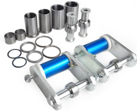
Rear frame bushings must be pressed in from the outboard side of the car, **Do Not** attempt installation from the inboard side; bushings will not go in from this direction. Grease fittings must be located on the inside of the frame. **Installation hint:** You can use all-thread ½ inch and a couple of heavy flat washers to facilitate frame bushing installation. Use the tool to pull the bushing into place in the frame rail. A large
