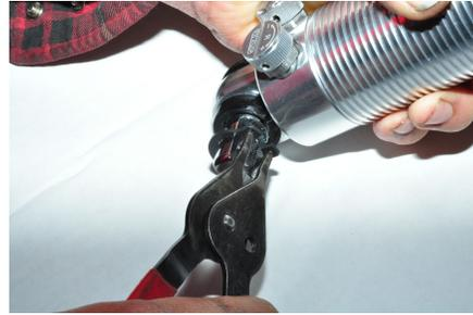
14. Remove the bar by tapping it out of the bushing with a dead blow hammer. If you have a small press you can use that.
