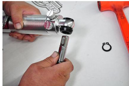
15. Next install the steel sleeve in the bushing, place grease inside the bushing and around the pin. We recommend synthetic grease like NEO Z-12, however any water resistant synthetic grease will work.
