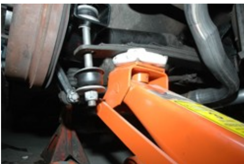
23. Lift the spring up by using a floor jack and slide the assembly through the hole.
