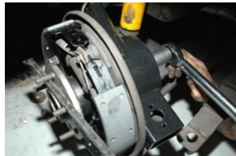
22. Install the spring cushion and bolts attaching the swing arm to the leaf.
