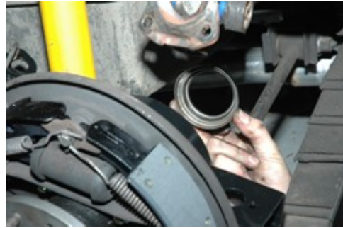
20. Install the axle shaft steel thrust washer, castle nut and torque to 120 foot-pounds. Install the axle 1/2 shaft and torque to 65 foot-pounds.
