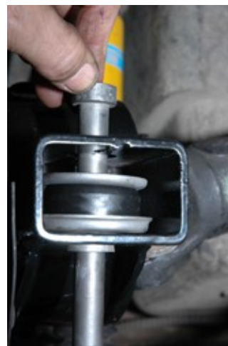
23. Lift the spring up by using a floor jack and slide the assembly through the hole.
