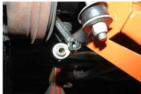
9. Next swing the strut rod up into the bearing hub. Make sure the 5/8-inch steel spacers are still in the rod end (one on each side of the rod end).
