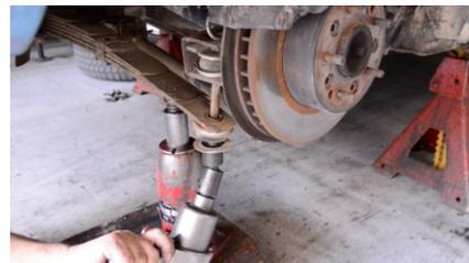
4. Next remove the nut and strut rod shock pin from the hub. The strut rod will drop out of the hub assembly. Do this to both sides.
