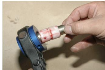
9. Install the thrust washers onto the bushing. One thrust washer on each side of the bushing. You need to slightly tap the thrust washers onto the pin.
