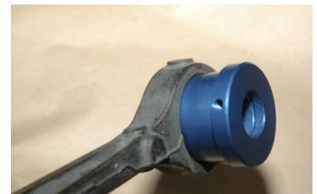
4. The next step will be to press the blue housing into the control arm. The bushing installs from the outside --- in. You will notice a small threaded hole in the edge of the bushing; this is for a grease fitting. Position the hole so that the fitting points towards the ball joint stud slightly down not even with the arm. This will allow you to lubricate the bushing once it is installed on the car.
