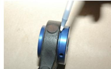
6. Once the press work is complete, lubricate the inside of the white insert with grease. We recommend using synthetic grease that is water resistant.
