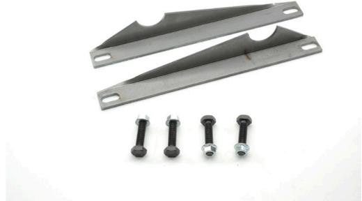
1. In your kit there will be two seat brackets. They attach to the rear seat bolts under neigh the car. We furnish the hardware in your kit. Locate (4) 10-mm bolts and nuts. Slide the front seats forward in order to remove both rear bolts holding the seat rails too the floor. Install the bolts supplied in the kit.
