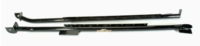
This kit requires welding the subframe to the unibody. We have designed both sides to self index. This makes placement simple. The 905-C does not require removal of the fuel lines or repositioning them. This installation will not interfere with exhaust or brake lines, nor will the interior need to be removed.
