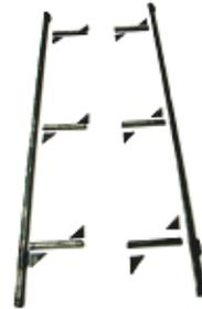
1. When installing 915 jacking rails, the main subframe 912 should be tack welded to the car in the front and rear. Do not weld them on yet. You are going to fit all the tubes (915 to the 912 kit) first, tack weld them together on the car, and then drop the subframe down and weld it complete before re-installing the assembly on the car.
