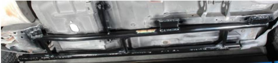
factory incorporated angle iron as part of the outer rail in order to add additional support. The 1-inch diameter rail will fit perfect inside the support.
