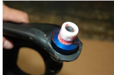
6. Install the plastic outer thrust washer and then the steel outer thrust washer.
