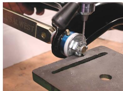
that of a wheel bearing cotter pin setup. Cotter pin each end of the shaft before installing on the car.
