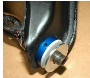
7. Install the slotted hex nut and tighten down the nut until there is thrust contact between the inner and outer thrust surfaces. You will run the nut to set the bushing and thrust washers. After they are seated, back off the nut and slightly tighten the nut down till you have thrust contact, then go 1/8 of a turn more or one flat on the nut. (You are adjusting the bushing as though it was a wheel bearing).
