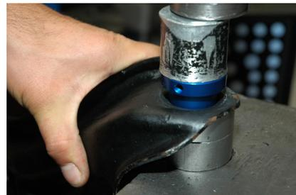
4. Next install the small steel thrust washers (one on each side of the shaft) first and then one of the small plastic inner thrust washers (one on each side of the shaft). Slide the shaft with the steel and plastic thrust installed through the upper arm bushing hole and into the bushing you just pressed in. Press in the bushing on the other side of the control.
