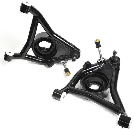
13. Slowly raise the arm to fit the ball joint into the spindle. Install the castle nut on the ball joint and torque to 90 ft-lbs. Next, tighten the nut to line up the slot in the nut and hole in the ball joint and install a new cotter pin.
