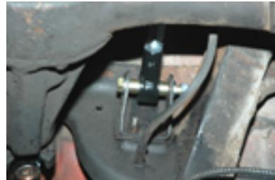
4. Next support the vehicle on jack stands under the rear end only and not the frame. Torque the bolt on the rear end side only after the car is resting on the suspension at ride height. Torque to 80 foot-pounds.
