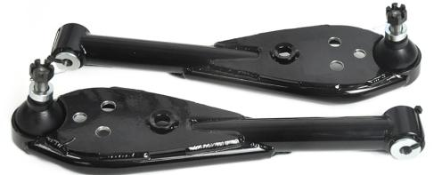
1. Raise and support the vehicle on the uni-body frame rails. Following a suitable service manual, remove the lower control arms. Notice the location of the lower control arm eccentric bolt. The eccentric directly effects the alignment. You may want to place a small mark on the eccentric and frame. When it comes to re-installation it will help getting the alignment closer from the start.
