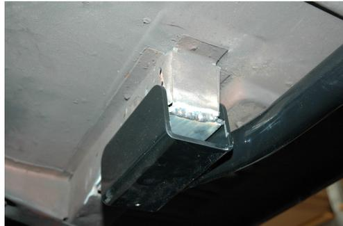
The back portion of the subframe will slide over the rear frame rail that goes over the differential.
