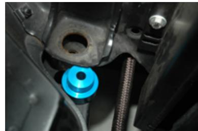
7. Install the female portion of the bushings located at the firewall and radiator core support. The bushing indexes on the step of the installed male bushing and sandwiches the frame. Basically when the assembly is tightened, the bushing halves will lock the frame in position so it cannot slip.
