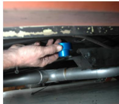
6. The final bushing on the passenger side is the radiator core support. It is one of the 2 -inch diameter male bushings with a 1/2 -inch hole. This bushing installs the opposite as the others. The step part of the bushing goes up through the radiator core mount. Slide the bushing into place and lower the body back down onto the frame.
