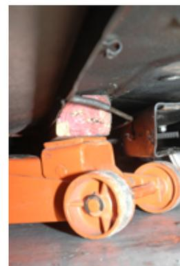
between the frame and body allow you to remove the old bushings and install the new.
