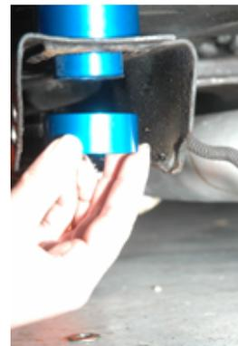
8. Install the female portion of the back bushing located with the subframe kit. Install using a 5/8 x 4-inch long bolt with a 5/8-lock washer and 5/8 flat washer. Do not tighten yet.
