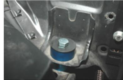
11. Once the bolts are all installed run them down a little. **DO NOT TIGHTEN.** They must have room to pivot because you have to do the other side.
