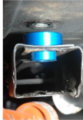
5. After completing step 4, install the 2-1/4-diameter bushing from the 809 kit at the firewall position.
