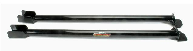
Installation of this kit requires the vehicle to be fully loaded on a drive on lift. The subframes will tuck up tight against the floor. No ground clearance will be lost. If you have side exhaust that exits before the rear tires, there is a good possibility the subframes will interfere. Normal exhaust routing will not be a problem.
