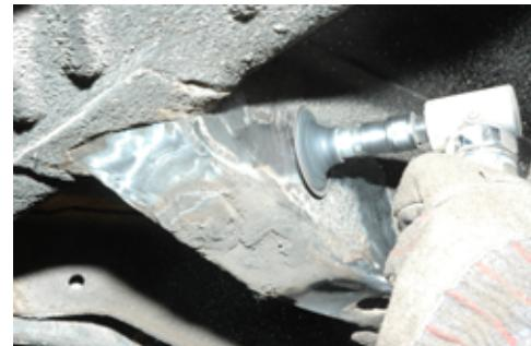
5. After you have prepped the frame and subframe. Hold the subframe up into position and tack the subframe to the frame rails. Make sure the forward portion of the subframe intersects the forward two rails and the subframe. Notice the subframe does not cover up the frame rail holes.
