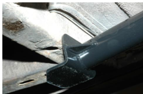
2. Just before the middle of the subframe you will have to grind (clearance / notch) a small portion of the seat bolt support rail that is welded to the floor. As you can see in the below photos there is very little material removal.
