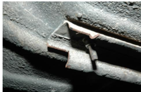
3. Once you finished notching the floor support, the subframe will go up tight against the floor rails. Push the subframe forward on the car so it butts up against the forward floor rail. Mark the floor
