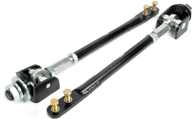
**Important: You should never have 5/8 of an inch or more of threads showing on the rod end side of the adjuster for two reasons: First it is unsafe, not enough threads holding the assembly together. 2<sup>nd</sup> You should never be in that position anyway because you would be setting negative caster. Negative caster creates wander and has no self-centering action.**
