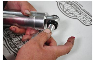
16. The steel sleeve will push into the bushing fairly easy. Push the sleeve in till it bottoms out with the bushing.
