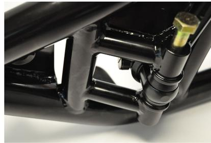
19. Next lift the lower ball joint up into the spindle. Install the castle nut on the ball joint and torque to 80 ft-lbs. Next, tighten the nut to line up the slot in the nut and hole in the ball joint and install a new cotter pin.
