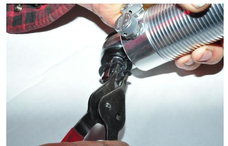
13. First remove the bar from the base of the shock. Almost all the shock companies make something similar. They have a c-clip on each side of the bushing.
