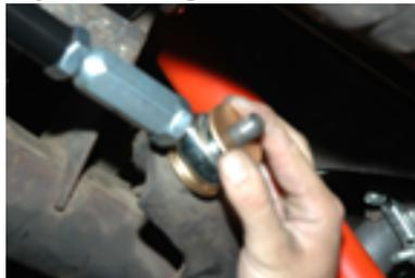
3. Place the lock washer and nut on the rear end stud and torque to 80 foot-pounds.
