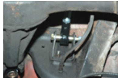
5. Check pinion angle: The pinion angle should be set with the vehicle at ride height on a drive on ramp. Measure the angle between the rear end and drive shaft. We recommend 2 to 3 degrees nose down. To adjust the angle, simply adjust the length of the upper control arm by using a one-inch wrench. Loosen the jam nuts first and then rotate the hex adjuster, by lengthening or shortening the upper arm will adjust the pinion angle. After the pinion angle is adjusted tighten the jam nuts.
