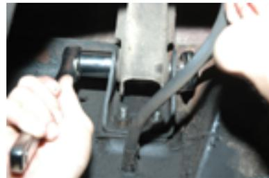
2. Install the new upper control arm with new hardware on the rear end side first. Install the new bolt with a flat washer against the head of the bolt and one against the lock nut. Tighten the bolt down till it contacts the bracket. Do not torque the bolt yet.
