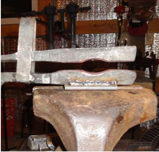
The “spring pipe fuller” jaws need to match the size of the pipe you will be forging. The width of the opening needs to be about 1.5 times the pipe diameter, and the height of the opening should be about one-fourth of the pipe diameter.
