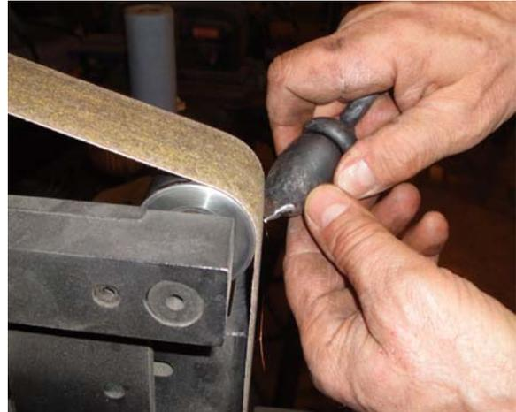
**Grind scale off the nut**
