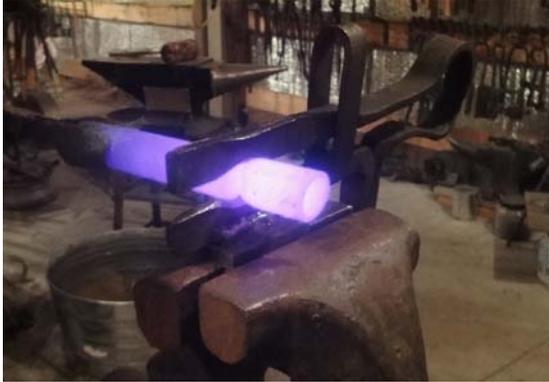
**Using the spring pipe fuller**
