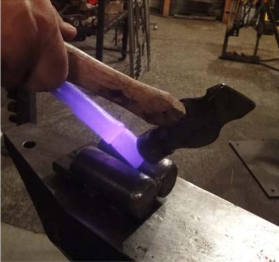
**Forge the nut tip down to nearly 1/4" diameter**
