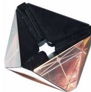
Figure 5 – Six triple-prism glass assembly.
